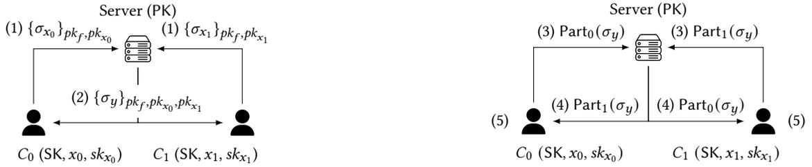
(a) Computation of  $y = f(x_0, x_1)$  where the function  $f$  is simulated by the server using PK over  $\sigma_{x_0}$  and  $\sigma_{x_1}$  the encoding of respectively the input  $x_0$  and  $x_1$ .
