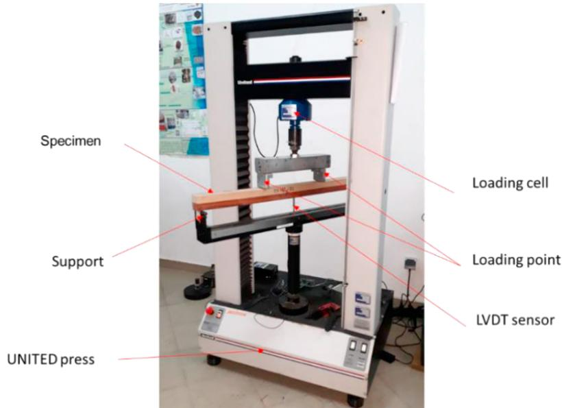
Fig 3: Experimental device
