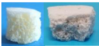
Figure 1: optical pictures of agelatin-bioactive glass foam before calcination (left) and a bioactive glass foam obtained after calcination (right)
