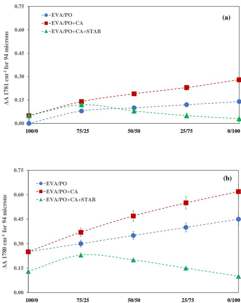
**Figure 4.** Variation in absorbance ( $\Delta A$ ) at  $1780 \text{ cm}^{-1}$  of EVA/PO, EVA/PO+CA and EVA/PO+CA+STAB after (a) 200 h and (b) 400 h of exposure to SEPAP 12.24/52 °C
