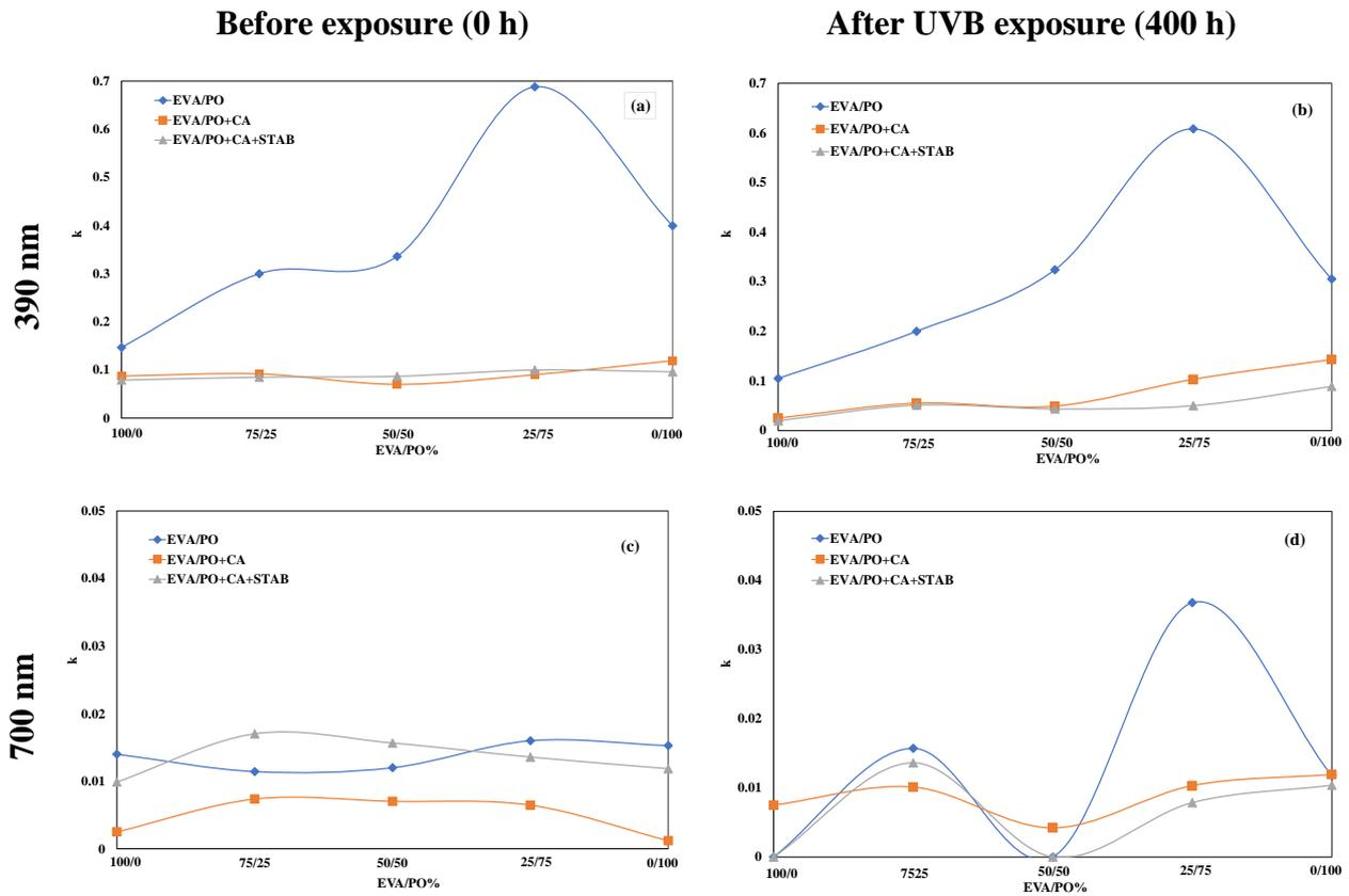
**Figure 6.** Linear attenuation coefficient,  $K$ , of EVA/PO, EVA/PO+CA and EVA/PO+CA+STAB under different conditions: (a) 0 h, at 390 nm, (b) 400 h, at 390 nm, (c) 0 h, at 700 nm, (d) 400 h, at 700 nm.
