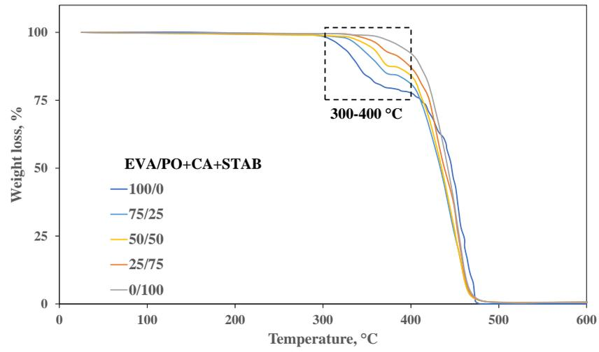
**Figure 2.** TGA curves of EVA/PO blends containing crosslinking agent (CA) and stabilizers (STAB)
