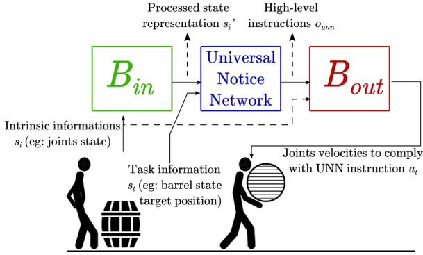
Fig. 3: UNN architecture. The agent receives an observation vector  $s$ , splitted into a robot observation vector  $s_i$  processed by the input base and a task observation vector  $s_t$ . The UNN, operates on the processed robot information and the task informations. Later the output base, computes the action based on UNN output  $c$  and robot intrinsic state vector  $s_i$
