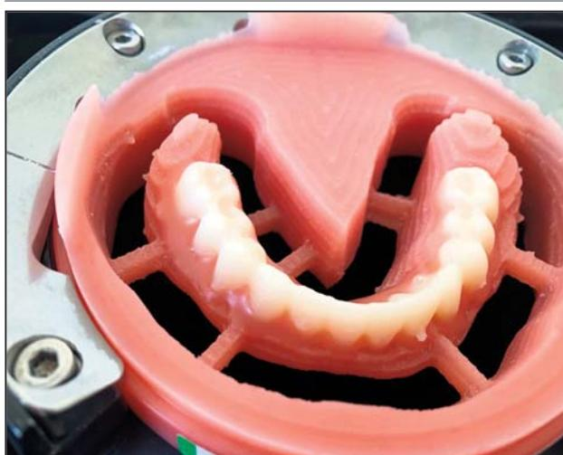
**Figure 5:** Computer assisted manufacturing of complete denture, using a milling machine
