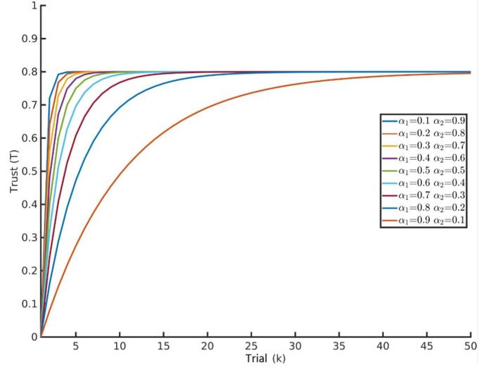
Fig. 2. Variation of Trust with parameter weights for a single task metric trust model. Performance is assumed to be constant i.e  $P = 0.8$ . The graph shows that even with constant performance the value of trust will increase with every trial and ultimately converge to the performance value.
