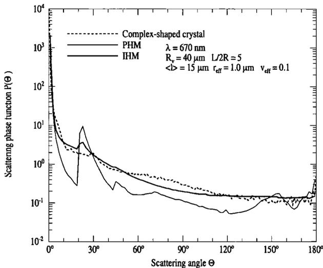
**Figure 1.** Comparison between different scattering phase functions.
