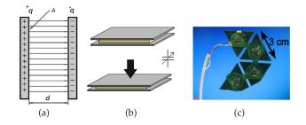
Figure 2: Capacitive Tactile Sensing Technology: (a) capacitance of a parallel plate capacitor depends on distance between plates d and area of the plates A (q is the stored charge) [45]; (b) two conductive plates are separated by an elastic dielectric – as force is applied, the distance between the plates reduces, changing the capacitance [9]; (c) mesh of triangle shape capacitive sensors for the palm of the iCub humanoid robot [44].
