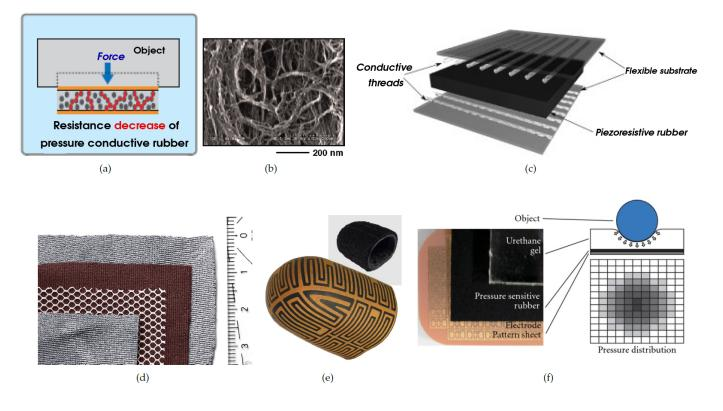
Figure 1: Piezoresistive Tactile Sensor Arrays: (a) illustration of resistance changes in conductive rubber [47],(b) nano-scale image of conductive rubber [48], (c) structure of piezoresistive tactile array [49], (d) piezoresistive fabric tactile sensor [50], (e) schematic of electrode layer of the 3D-shaped tactile sensor [34], (f) tactile image of a piezo-resistive pressure sensor array [35].
