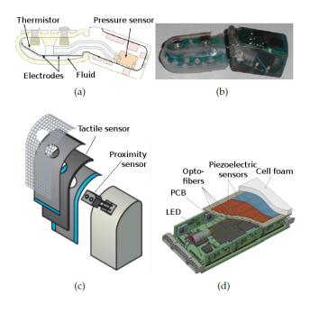
Figure 7: Multimodal Tactile Sensors: (a) schematic of the biomimetic BioTac tactile sensor with 19 electrodes, fluid pressure sensor and thermometer [84], (b) photo of the multimodal BioTac tactile sensor, (c) combined tactile-proximity sensor that can measure both the distance to an object and the contact pressure [90], (d) drawing of a multi-modal tactile sensing module consisting of optical and piezoresistive sensors [76].
