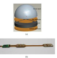
Figure 4: Quantum Effect Tactile Sensing: (a) structure of a tactel of the QTC based tactile sensing array with capability of measuring shear and normal forces [72]; (b) the flexible tactile sensing array for a finger of an anthropomorphic robot hand with the tactels that can measure shear forces [72].
