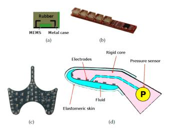
Figure 6: Sensors based on barometric measurements: (a) the structure of a tactile sensing cell with a barometer and silicon rubber (b), the TakkStrip tactile array of these cells [87], (c) custom shaped array of the pressure sensing barometers of the iHY hand [42], (d) micro-vibration sensing system based on a fluid pressure sensor of the BioTac tactile sensor [83].
