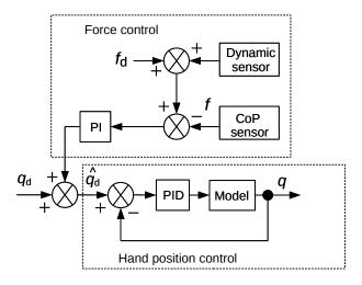
Figure 25: Block diagram of position-based force control using tactile sensors [39]. The position of a hand is modified according to the measured force and detected slip signal. The slip signal increases the desired force.  $q_d$ ,  $\hat{q}_d$ , and q are the desired joint angle, modified desired joint angle, and actual joint angle, respectively.  $f_d$  and f are the desired and actual forces. The desired force increases when the dynamic sensor detects vibrations.
