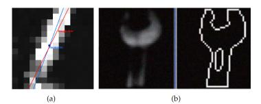
Figure 22: Contact pattern recognition and feature extraction from a tactile image: (a) extracted feature of contact edge based on image moments (blue line) and hough line transform (red line) [31]; (b) geometrical shape derived from the tactile image: original tactile image on the left and detected contour on the right [133].
