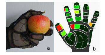
Figure 13: Tactile data glove based on conductive rubber (a) and the tactile information from the data glove during a grasp (b) [54].
