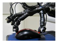
Figure 27: Hand with ellipsoid f/t sensors following a surface (the red dashed line) [104].
