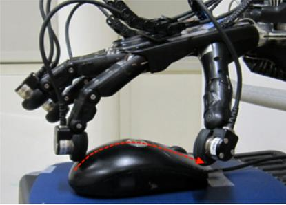
Figure 27: Hand with ellipsoid f/t sensors following a surface (the red dashed line) [104].
