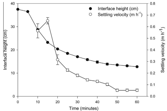
**Fig. 2.** Changes in the position of the interface height between the clarified medium and the settling biomass and settling velocity over time of a 10-day old N stressed *Arthrospira* batch culture in a 1 L Imhoff cone over the course of 1 h.
