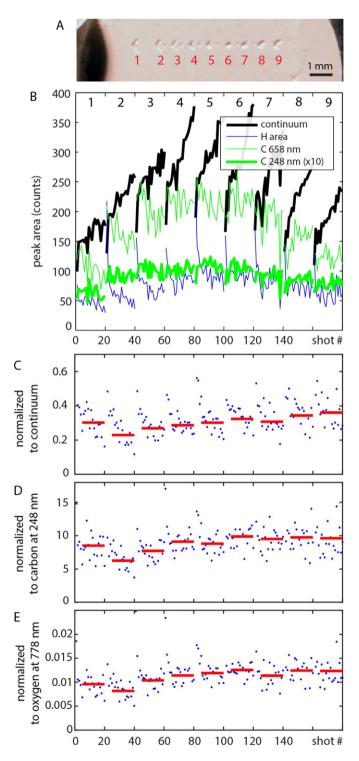
**Fig. 5.** Peak area shot-to-shot series for hydrogen and carbon (B) when varying laser focus during tests on a bassanite pellet in the laboratory (A). The sequence represents 9 points of 20 shots each. The single shot hydrogen signal (blue dots) and point-to-point average without 5 first shots (red) are represented with normalization to continuum (C), carbon at 248 nm (D) and oxygen at 778 nm (E).
