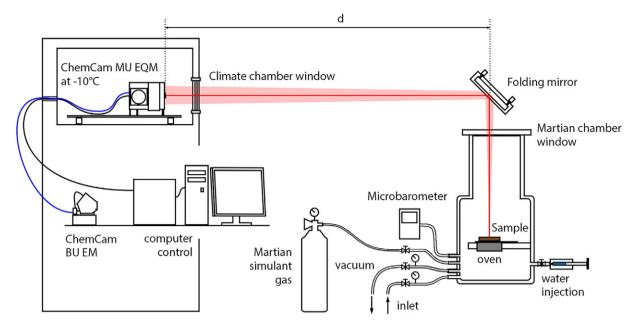
Fig. 1. Schematic of the ChemCam replica setup used for LIBS calibration in the laboratory.
