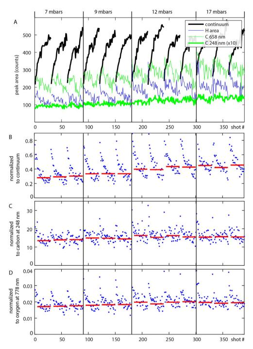
Fig. 6. Peak area shot-to-shot series for hydrogen and carbon (A) when varying CO<sub>2</sub> pressure from 7 to 17 mbar during tests on a bassanite pellet in the laboratory. The sequence represents 13 points of 30 shots each. The single shot hydrogen signal (blue dots) and point-to-point average without 5 first shots (red) are represented with normalization to continuum (B), carbon at 248 nm (C) and oxygen at 778 nm (D).
