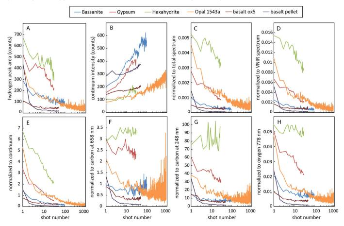
Fig. 11. Shot-to-shot profiles of the hydrogen signal for several types of samples containing homogeneous water content and showing decrease of the hydrogen signal count (A). On the other hand, the continuum intensity shows continuous increase (B). Results using the different normalizations of the hydrogen signal are shown in plots C to H.
